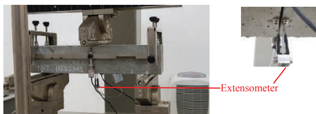
Figure 1. Three-point bending test of HPC beam notched incorporating nano - silica
