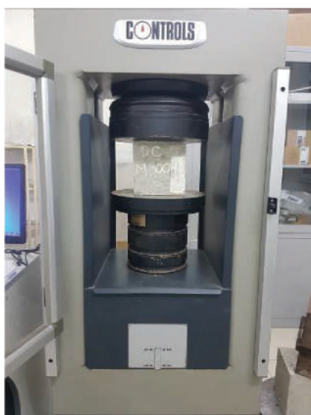
Figure 3. Advantest 9 system at Construction Laboratory, HUMG
