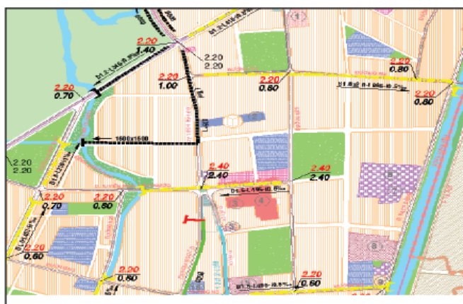
Figure 3. The all roads are designed with the same height and slope of less than 1% Tra Vinh City area [5]
